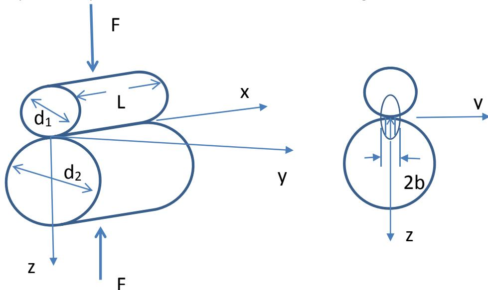
We are interested in calculating the magnitude of the principal normal stresses ( $\sigma_x, \sigma_y, \sigma_z$ ) and maximum principal shear stress ( $\tau_{max}$ ) in the larger cylinder for points beneath its surface, i.e. for increasing values of  $z$ . These may be calculated as follows<sup>1</sup>:
